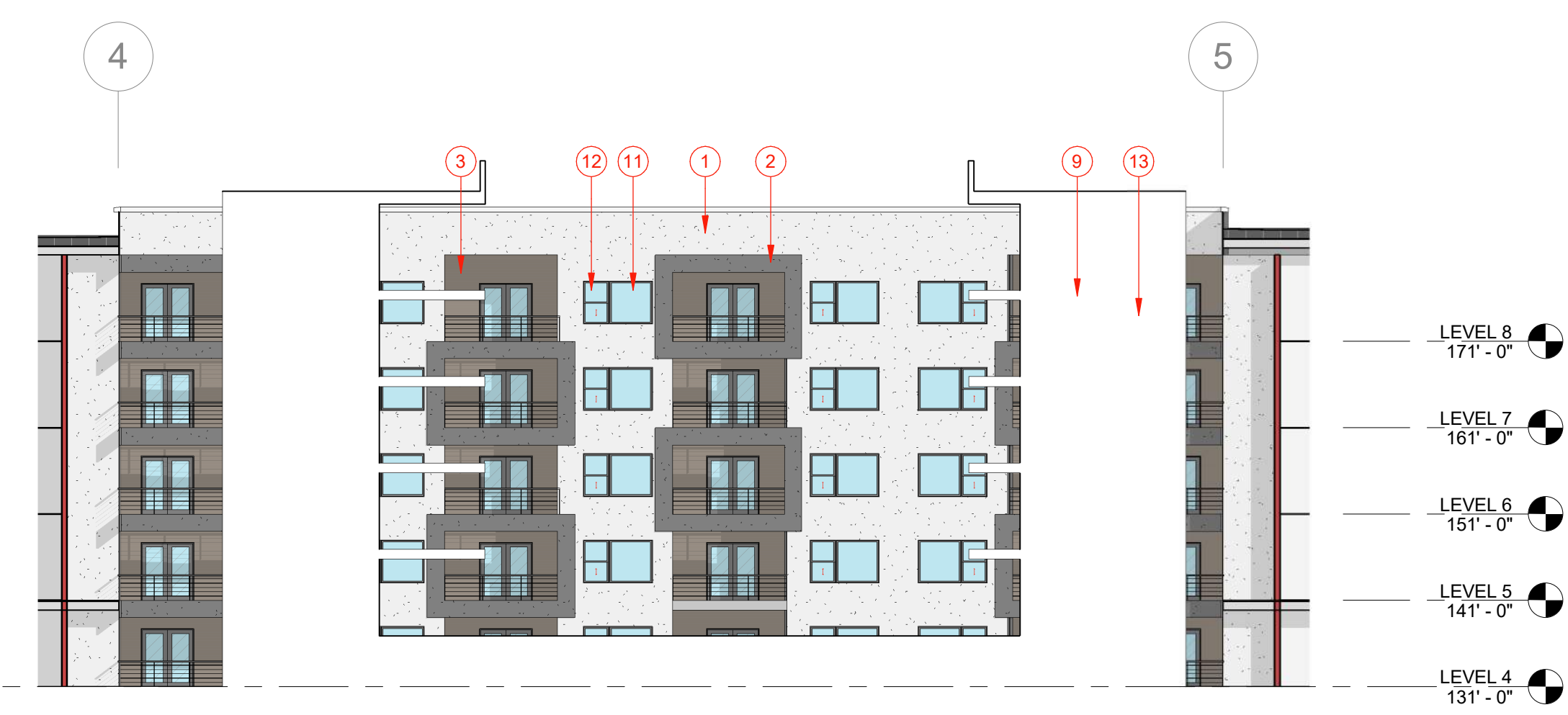
2 COURTYARD 01 NORTH ELEVATION. 1/16" = 1'-0" 0' 8' 16' 32'
