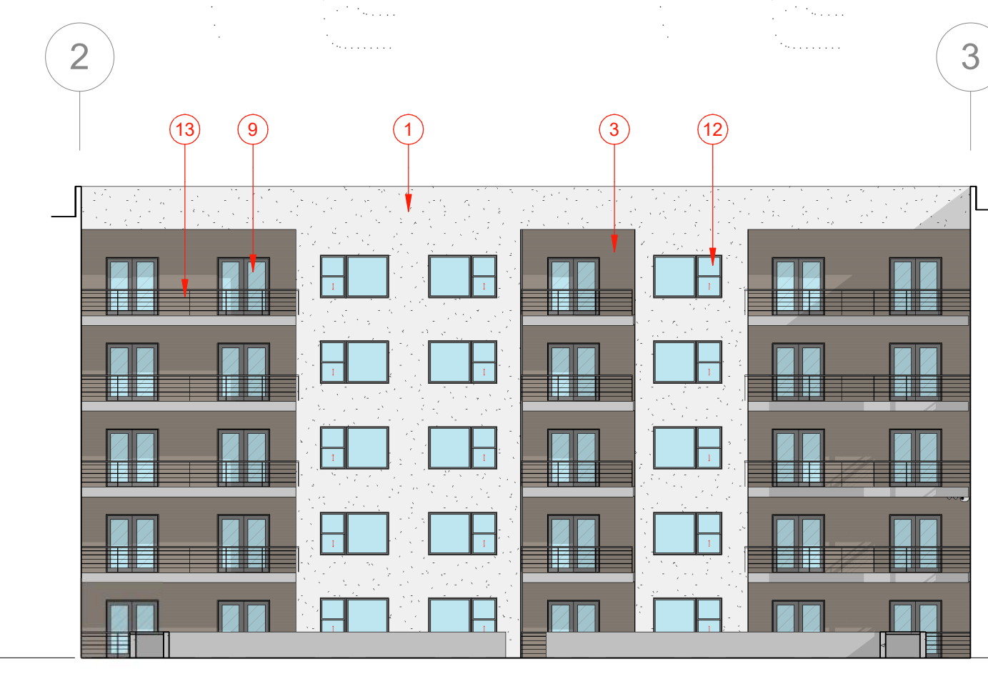
5 COURTYARD 02 NORTH ELEVATION. 1/16" = 1'-0" 0' 8' 16' 32'
